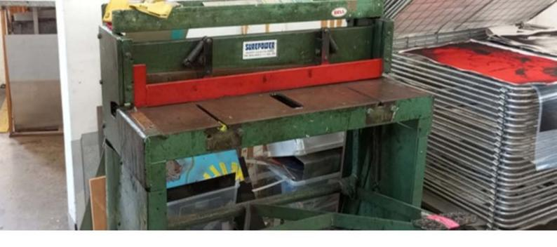
This is the manual guillotine which is used for cutting metal plates. I can ask for assistane if I find it difficult to use. It will make some noise when in use.
